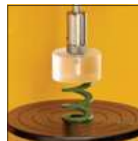
TA-11 Spring Rate Test measures force vs distance of springs
