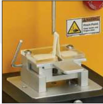
TA-KF F Kieffer Dough and Gluten Extensibility Fixture quantifies maximum force and distance needed to break sample. Fixture Base Table required.
